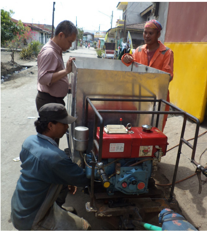
A model of mobile desludging equipment that designed to reach narrow village lanes in Medan Belawan.
